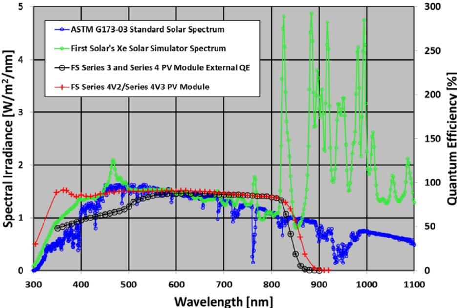
Figure 3. Comparison of the ASTM G173-03 standard solar spectrum and First Solar’s continuous xenon arc solar simulator spectral output. The external QE data from Figure 1 are included for reference, and indicate that good agreement exists between spectral irradiance distributions over the response range of First Solar PV modules.
