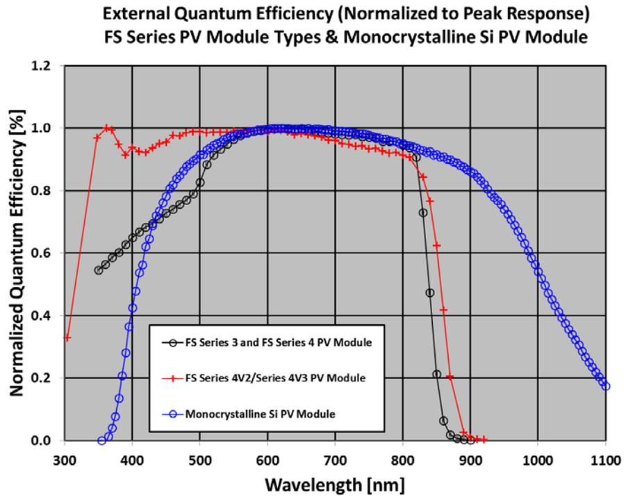
Figure 2. Normalized external quantum efficiency of First Solar FS Series 3, FS Series 4, and FS Series 4V2/Series 4V3 CdTe PV Module types, compared with that of a monocrystalline Si PV module.
