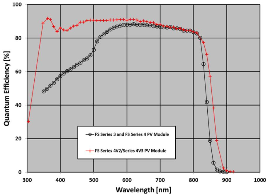
Figure 1. External quantum efficiency of a First Solar FS Series 3, FS Series 4, and FS Series 4V2/Series 4V3 PV Module types.
