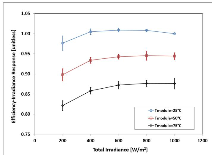
Figure 2. Dependence of  $P_{MAX}$  on total irradiance and module temperature for S4V2 modules. This is a representation of the response of S4V2 modules with an 110W nameplate power.
