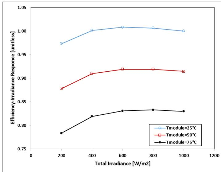
Figure 3. Dependence of  $P_{MAX}$  on total irradiance and module temperature for S4V3 modules. This is a representation of the response of S4V3 modules with an 117.5W nameplate power.
